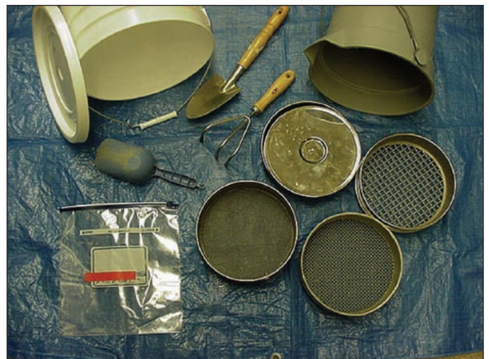
Figure 6. Materials needed to collect a composite sample.
