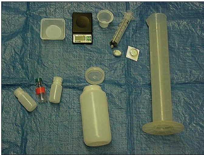
Figure 4. Most of the equipment and materials needed to leach a sample using the Field Leach Test.
