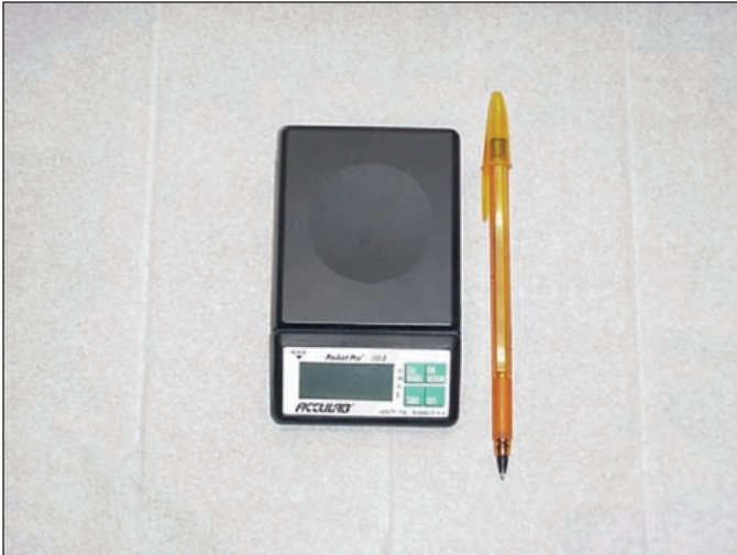
Figure 5. Close-up of small field balance that can be used to weigh sample for leaching on-site using the U.S. Geological Survey Field Leach Test.
