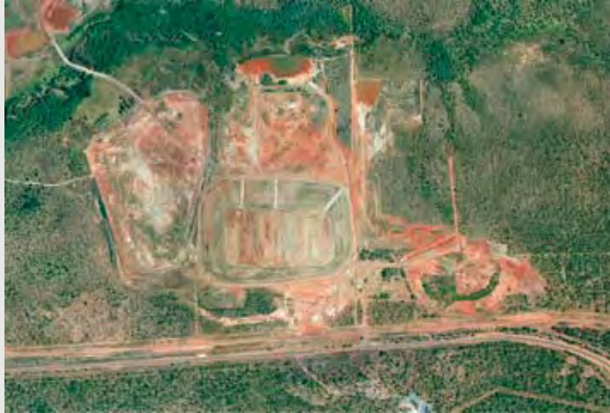
Figure 4: Rehabilitated mine site in 2005, following construction of cover over the waste rock pile, with revegetation to be completed
