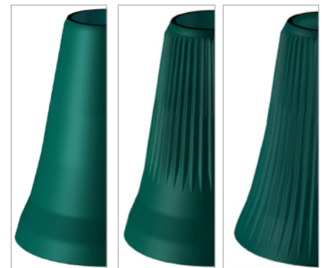
Examples of smooth (left), partially corrugated (center) and fully corrugated (right) mantle profiles.
