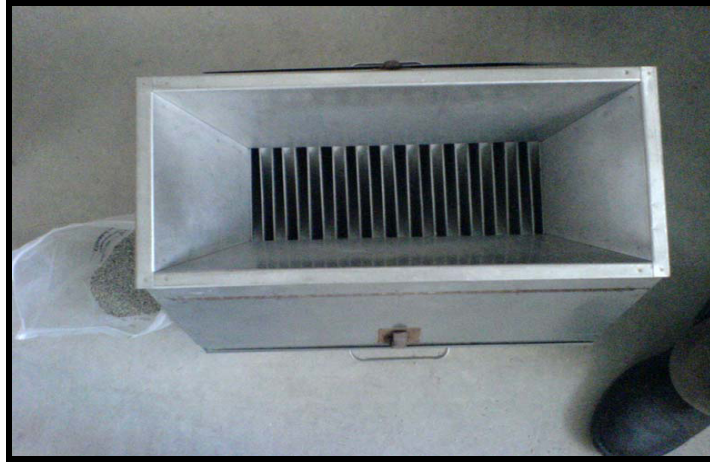
Figure 2.14 Typical chute riffles.
