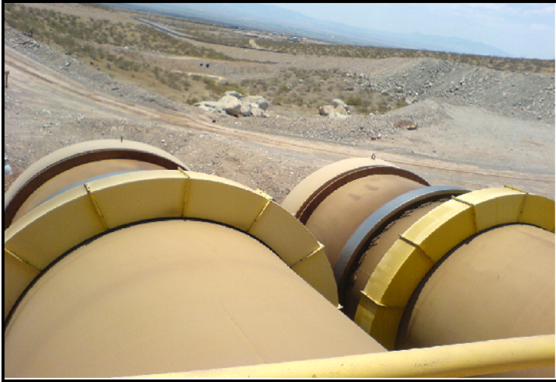
Figure 3.3 Agglomeration drums at a copper heap leach operation.
