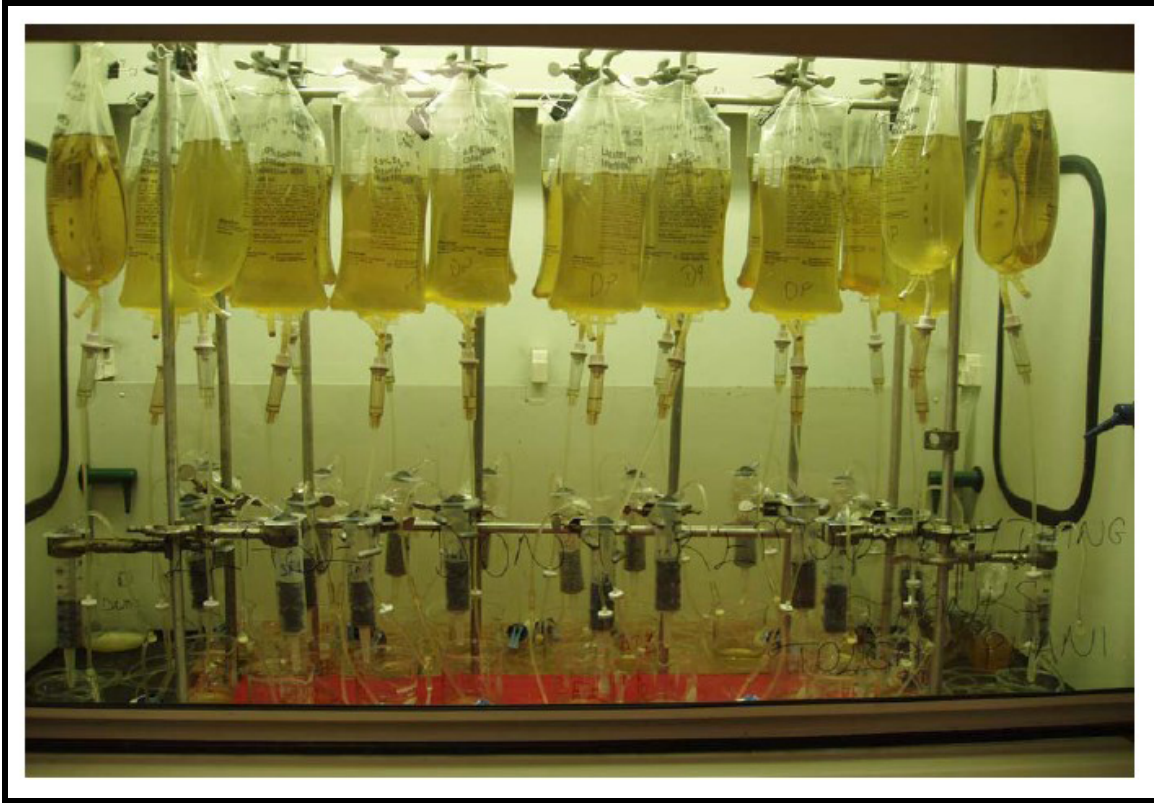
Figure 2.16 Laboratory column leaching setup showing IV irrigation and disposable syringe bodies containing ore samples.
