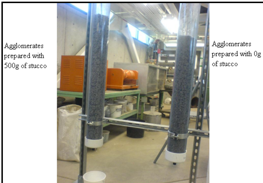
Figure 3.10 Columns loaded with agglomerates. Note the bulk density change. The agglomerates prepared with stucco binder filled the column to height 5 inches greater than the height without stucco binder.
