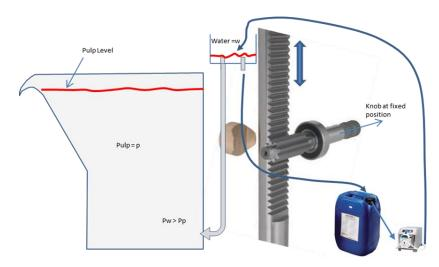
2. Changes in Froth Recovery (Fr): when you change the froth bed height, you are indeed changing the froth recovery and therefore the overall cell recovery from the following, where  $R_{flot}$  is the flotation recovery and Rc is the lab collection zone recovery  $Rc = (1 - \exp(-kt))$ . Rmax. You can determine froth recovery by doing a few froth bed heights and extrapolating to zero height.
