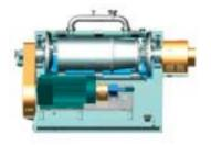
Feed slurry is introduced into the bowl through the centre of the conveyor where the solids settle through the liquor pool formed in the bowl. The gearbox produces a slight differential speed between the rotation of the bowl and that of the screw conveyor which conveys the solids along the bowl wall, out of the liquor pool, and up the conical section of the bowl to the solids discharge ports.
